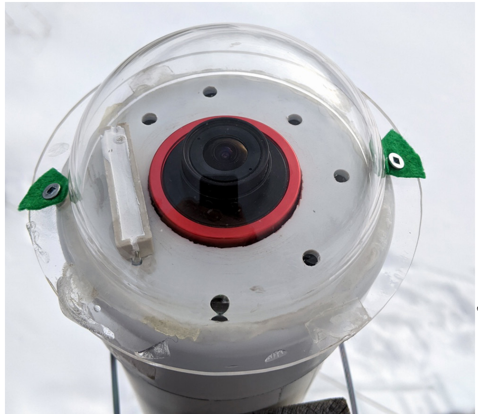
The dome heater with a silicon bead between the dome and the lid with vent holes in the lid to the housing - Kevin Kell
