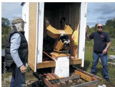
May 25: Here is the fork on the pier. They nicely fit into the new observatory building. The next job will be getting the scope onto the fork, and then getting the electronics going.
