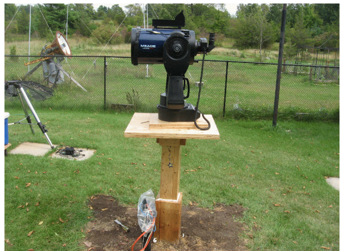
The pier was lowered, a platform and mount was built and the scope attached. Power and usb services come in from the bottom conduits.
