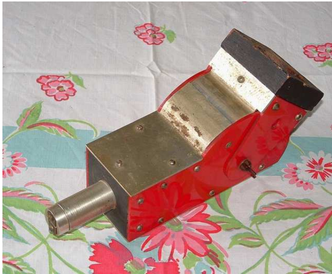
The small spectroscope. The small tube at left fits a 1.25" focuser.
