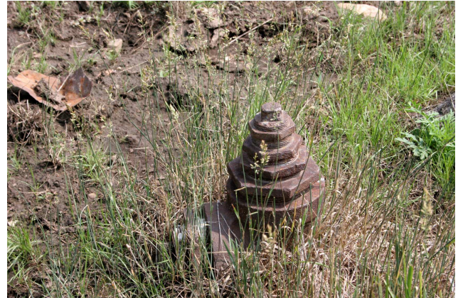
The cap from drill hole #1. Earlier seismic and gravimetric tests supported the impact crater hypothesis, which was confirmed through the drilling program. The bit at hole #1 jammed and broke, and still remains 1128 ft down.
