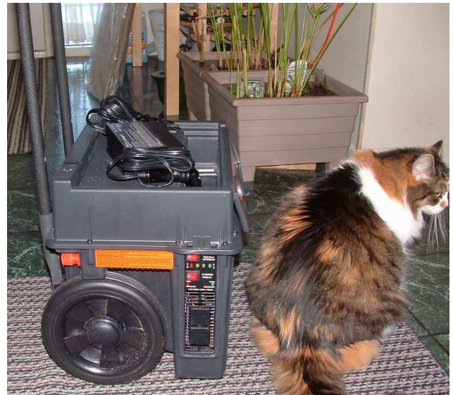
Side of the unit with a battery test button on top and the power switch for the AC inverter underneath it. Photo by Kevin
