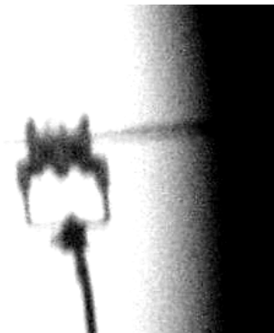
Same object, telescope and eyepiece but taken at the edge of the field. Details are lost because of telescope and eyepiece aberrations.
