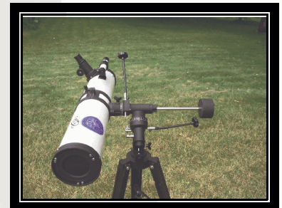
11cm f7.9 Orbitor Equatorial purchased in 2000 25mm(x36) kelner, 15mm(x60) kelner, 9mm (x100) kelner
