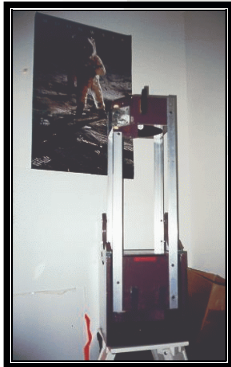
20cm f4.5 Barney Dobsonian built in 1999 8mm B&L plossl (x51), 30mm B&L plossl (x30)
