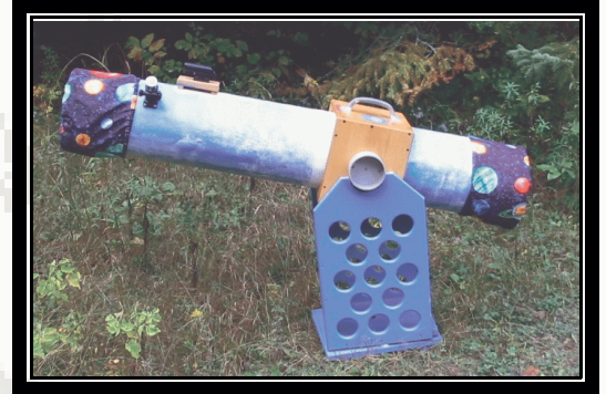
20 cm f7 Fitzgerald Dobsonian built in 1997 25mm RKA (x55)
