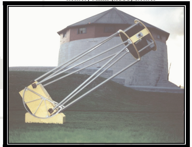
61cm f4.56 Venor Dobsonian built in 2002 32mm Erfle Focus Scientific 2003 (x88) 18mm Orthoscopic University Optics 2003 (x157) 12.5mm Orthoscopic University Optics 2003(x223) 2x Barlow Televue 2003
