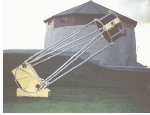
The 61 cm Venor Dobsonian-Mount telescope.
