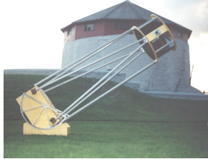
The 61 cm Venor Dobsonian-Mount telescope.
