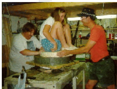
Grinding the 24" using a suitable mass
