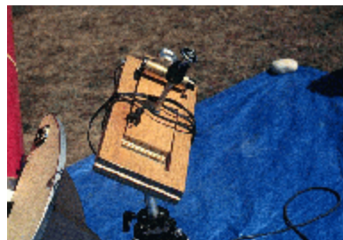
A double arm barn door tracker design from StarFest '98. One of the designs we are looking at using on the Mark II Barn Door Tracker project.
