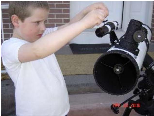
*Ivor Benderavage identifies two of four alignment screws for the finderscope of an "Orbitor" telescope.*
