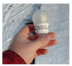
The light output dropped over 5 times, yet still fulfilled the function of navigation aids.
