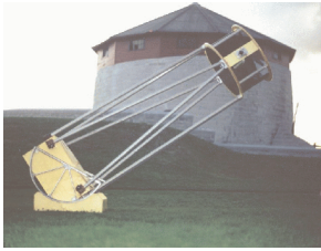
The 61 cm Venor Dobsonian-Mount telescope.
