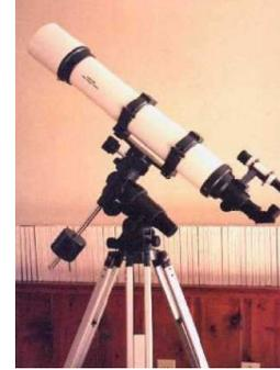
Advantages: Refractors, by default, have a totally clear aperture. No central obstruction causes light to be scattered from brighter to darker areas. Thus, contrast is good in refractors. Refractors are often chosen as the premier instruments for planetary and double-star observing. Refractors are also low in maintenance.
